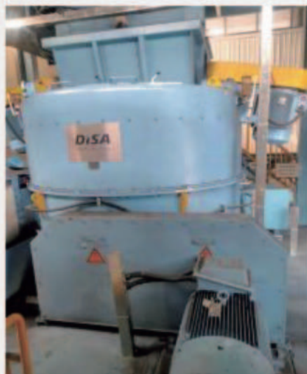
混砂机 / Sand mixing machine
